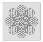
Basic properties of wire ropes 8x19W - IWRC are similar to the ones of ropes with fibre core and of the same structure.
